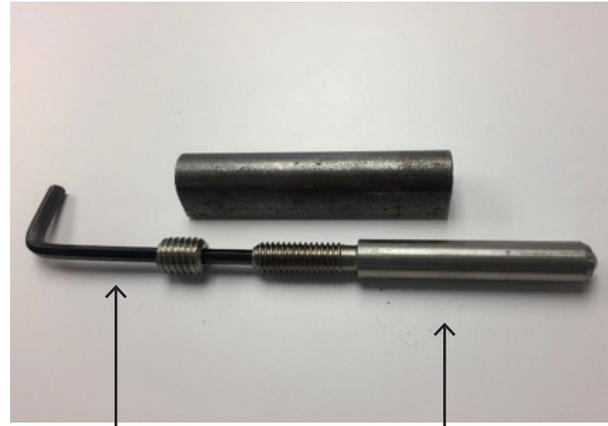
5mm Allen key shown inserted through hollow locking grub screw
