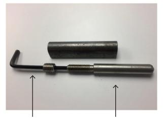
5mm Allen key shown inserted through hollow locking grub screw
