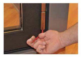
To adjust in height loosen the lock nut with a 6mm Allen key.
